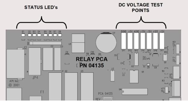
Figure 6-22. Location of relay board Status LEDs
