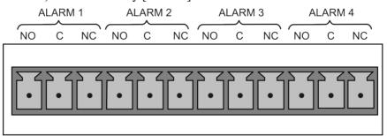
Figure 2-11. Concentration Alarm Relay
