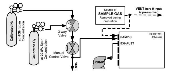
Figure 4-4. O<sub>2</sub> Sensor Calibration Set Up
