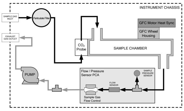
Figure 2-30. T300/T300M Internal Pneumatics with CO<sub>2</sub> Sensor Option
