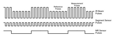
Figure 6-16. Segment Sensor and M/R Sensor Output
