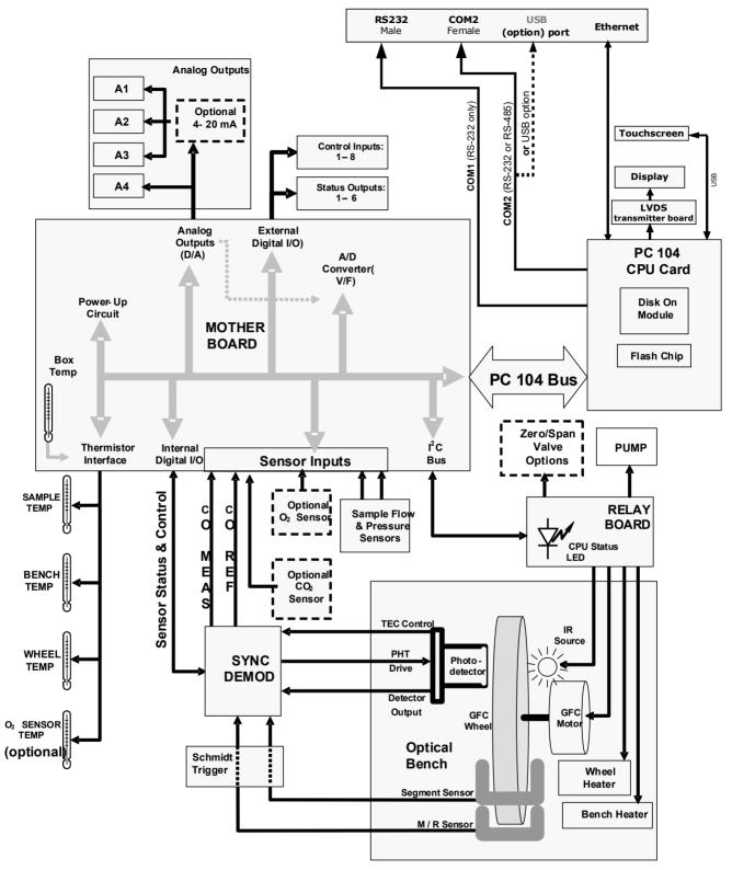
Figure 6-12. T300, T300M Electronic Block Diagram
