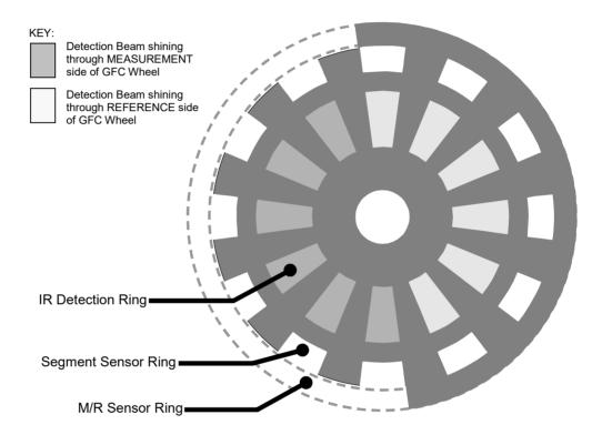
Figure 6-15. GFC Light Mask
