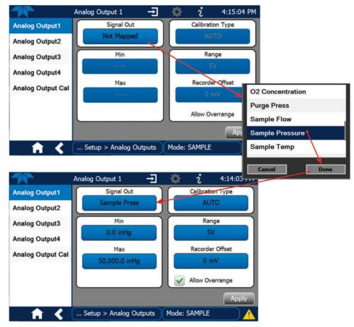
Figure 2-54. Analog Output Configuration Example
