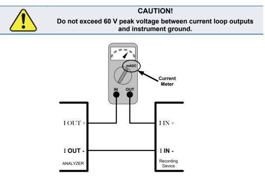
Figure 2-58. Setup for Checking / Calibration Current Output Signal Levels
