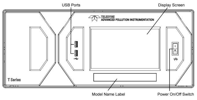
Figure 2-1. Front Panel Layout
