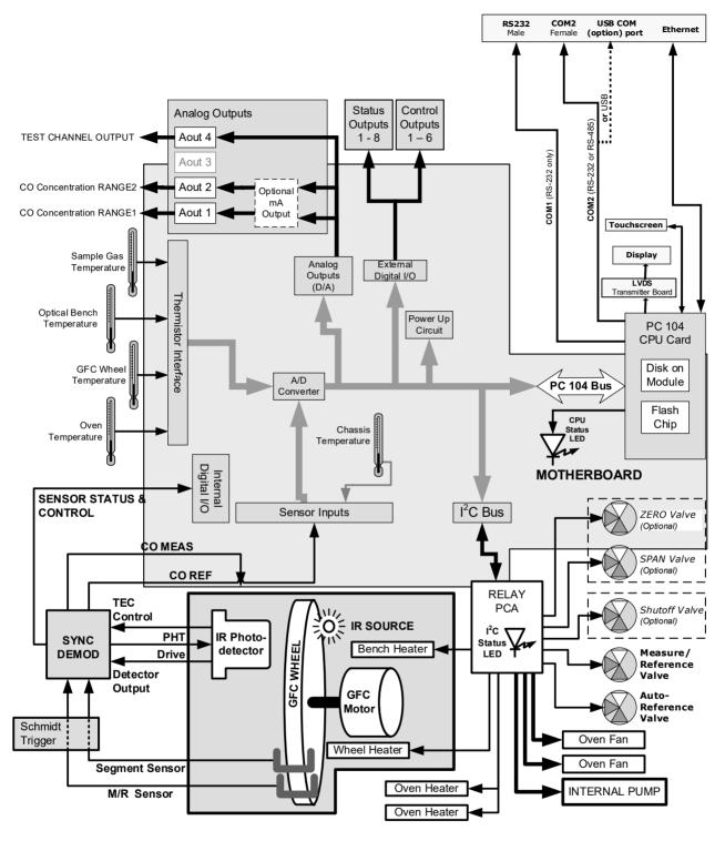
Figure 6-13. T300U Electronic Block Diagram
