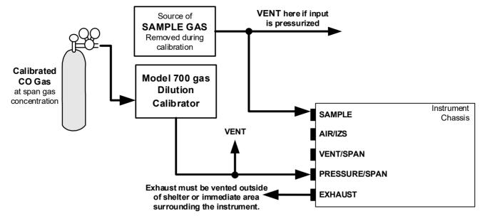
Figure 2-21. T300 Pneumatic Connections – Option 50H: Zero/Span
