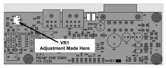
Figure 5-18. Location of Sync/Demod Gain Potentiometer
