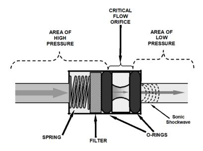
Figure 6-10. Flow Control Assembly & Critical Flow Orifice
