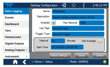
Figure 2-42. Datalog Configuration, Existing Log
