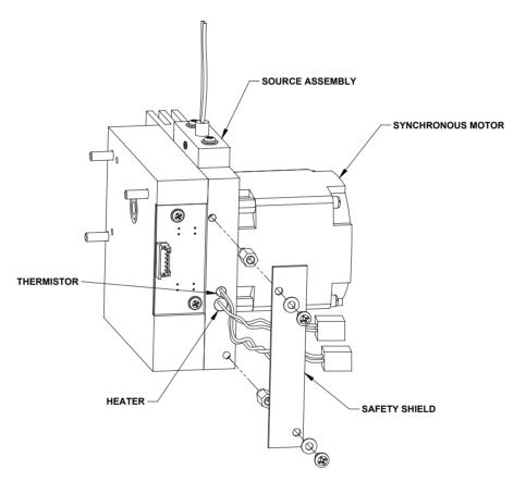
Figure 5-13. Opening the GFC Wheel Housing
