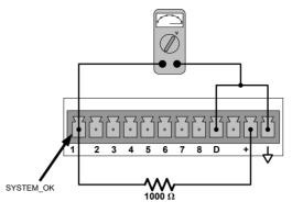
Figure 5-10. Typical Set Up of Status Output Test
