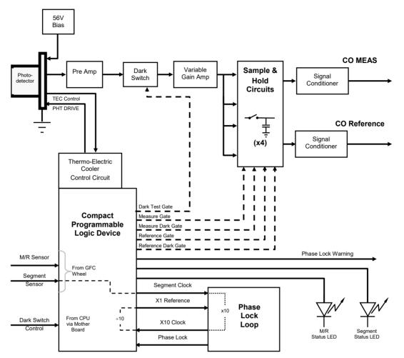
Figure 6-17. T300/T300M Sync/Demod Block Diagram
