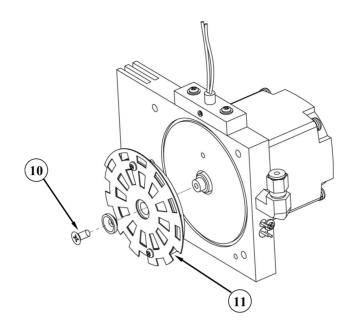
Figure 5-16. Removing the GFC Wheel
