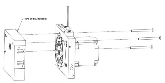
Figure 5-15. Removing the GFC Wheel Housing
