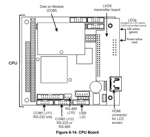
The CPU includes two types of non-volatile data storage: a Disk-On-Module (DOM) and an embedded flash chip.
