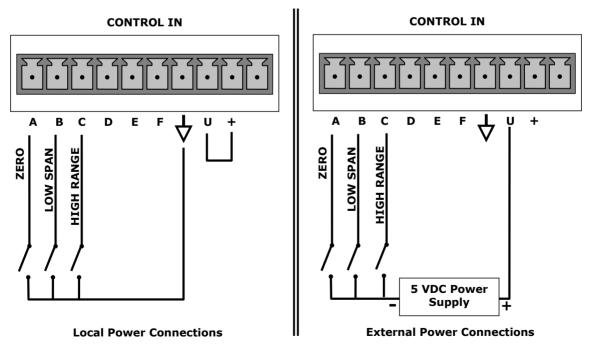
Figure 2-10. Control Input Connector
