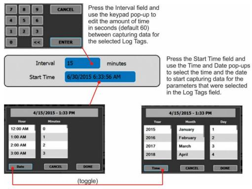
Figure 2-44. Datalog Periodic Trigger Configuration
