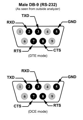
Figure 2-12. Rear Panel Connector Pin-Outs for RS-232 Mode
