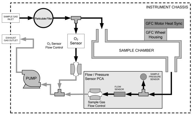
Figure 2-29. T300/T300M Internal Pneumatics with O<sub>2</sub> Sensor Option
