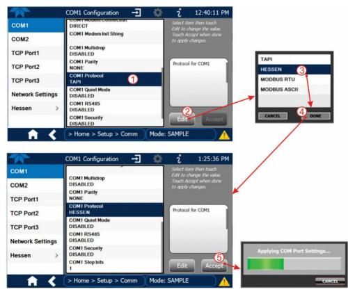
Figure 3-3. Serial Communication, Setting Hessen Protocol
