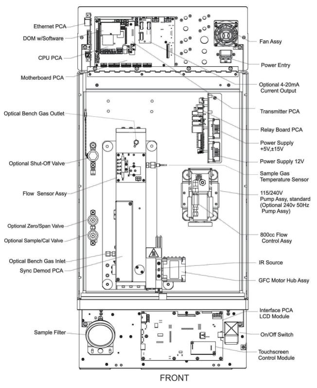
Figure 2-4. Internal Layout – T300M
