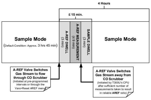
Figure 6-8. Auto-Reference Measurement Cycle
