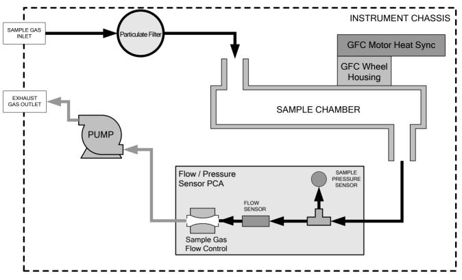
Figure 6-9. Internal Pneumatic Flow – Basic Configuration
