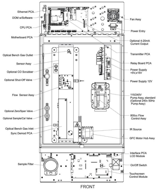
Figure 2-3. Internal Layout – T300
