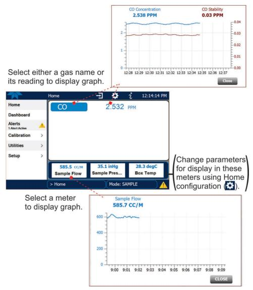
Figure 2-36. Concentration and Stability Graph (top) and Meter Graph (bottom)
