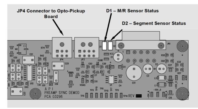
Figure 5-8. Sync/Demod Board Status LED Locations
