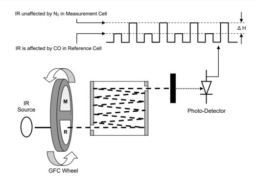
Figure 6-3. Measurement Fundamentals with GFC Wheel
