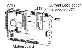
Example setup: install jumper shunts for voltage output on J19 and J23; remove jumper shunts and install Current Loop option for current output on J21.
