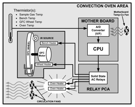
Figure 6-19. T300U Heating Control Block Diagram
