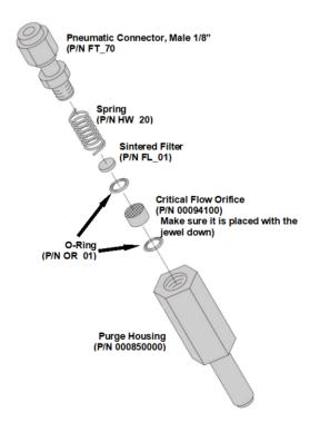
Figure 5-12. Critical Flow Restrictor Assembly/Disassembly
