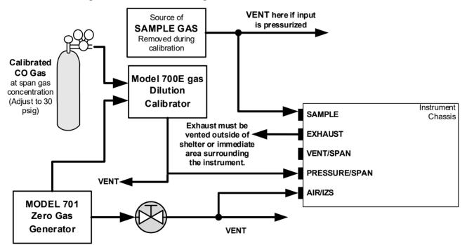
Figure 2-18. T300/T300M/T300U Pneumatic Connections – Option 50A: Zero/Span
