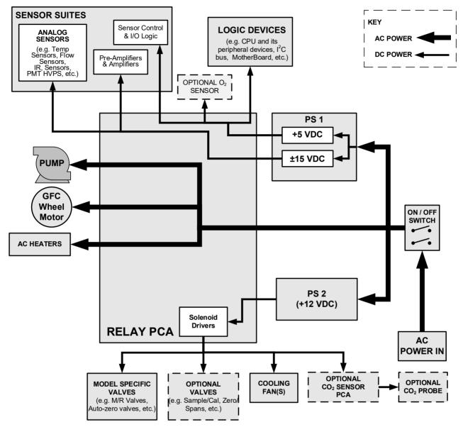
Figure 6-23. T300, T300M Power Distribution Block Diagram
