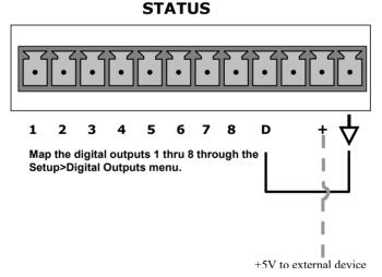
Figure 2-9. Status Output Connector for Digital Outputs
