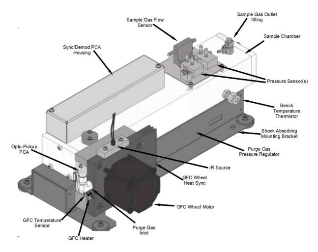
Figure 2-6. Optical Bench Layout (shorter bench, T300M, shown)
