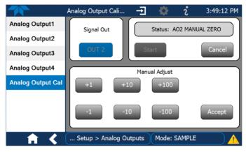
Figure 2-56. Analog Outputs Manual Calibration Screen (AOUT2 Example)
