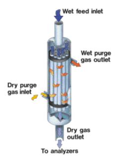
Figure 6-11. Semi-Permeable Membrane Drying Process
