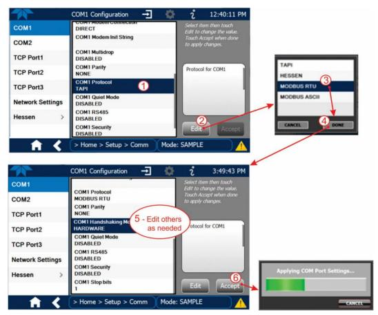
Figure 3-2. MODBUS via Serial Communication (example)
